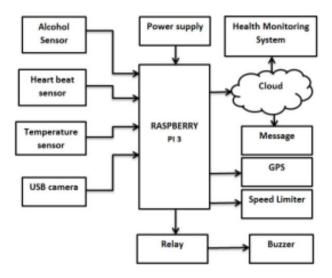
Fig. 2. Block diagram of IOT based driver drowsiness detection and health monitoring systems [9]
