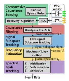
Fig. 1. Block diagram of the proposed heart rate tracking method [8]
